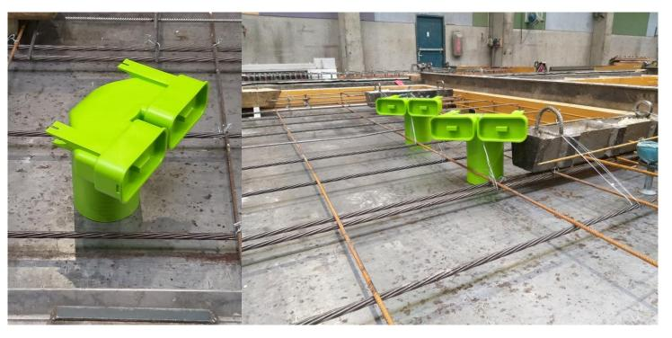
Valve adapter(s) placed over magnet on metal floor plate
