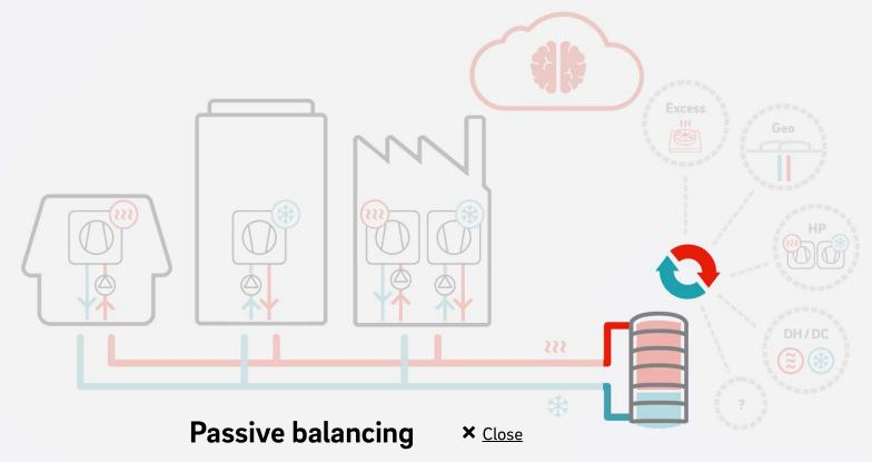
A water storage tank balances the warm and cold water levels, maximizing the re-use of energy in the grid. New energy can be supplied at the right moment from intermittent, renewable sources.
